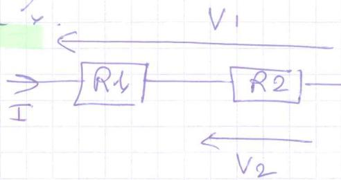
$$I = \frac{V_1}{R_1 + R_2}$$
